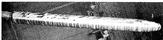
Fig. 25 Surface oil-flow pattern, M = 0.8 , \alpha' = 72^\circ , R_{ed} = 2.03 \times 10^6 (side view).
